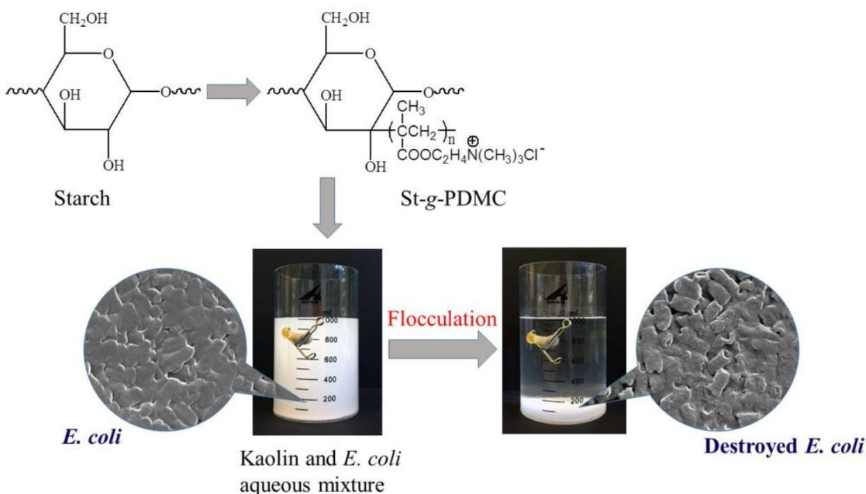
Fig. 1. Simultaneous removal of turbidity and inhibition of *E. coli* in water using a graft starch flocculant.
