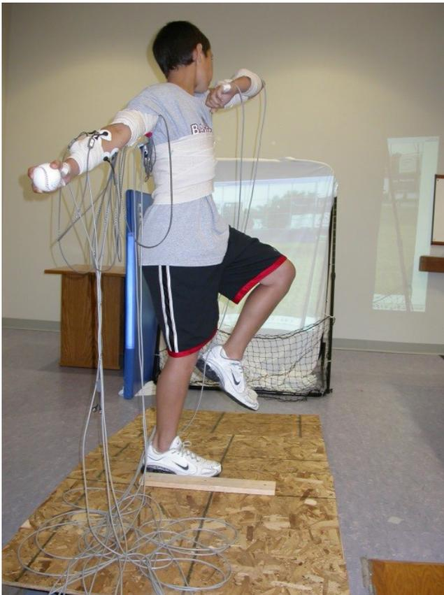
Fig. 1. Wired electromagnetic markers are used to record kinematic data as the pitchers throw into a pitching net.
