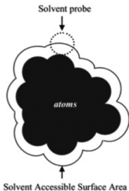
Fig. 1. The dark central area, composed of atoms, can be thought of a 3D protein and the outline around that area can be thought of accessible surface area that area.
