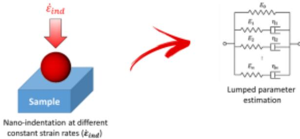
Fig. 2. Schematic of the nano-epsilon dot method. Samples are tested through nano-indentation measurements at different constant strain rates ( $\dot{\epsilon}_{ind}$ ). The results are used to derive viscoelastic constants (i.e.  $E_i$  and  $\eta_i$ ) for lumped parameter models.
