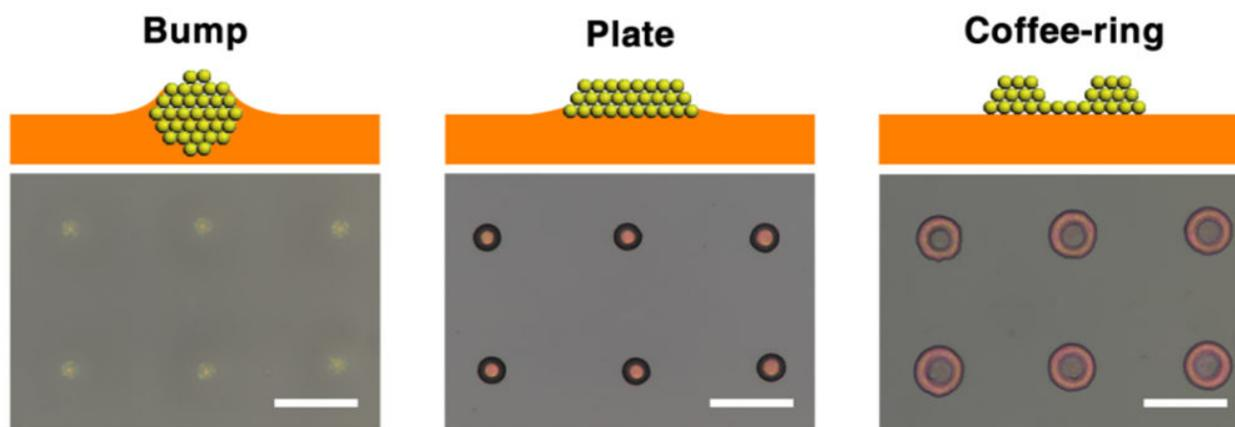
Fig. 1. Three kinds of PC dots shaped as bump, plate and coffee-ring, respectively.
