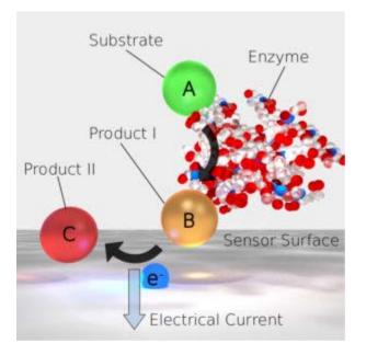
Fig. 1. Illustration of one possible detection mechanism. The enzyme moves freely in liquid while continuously catalysing substrate molecules A into product molecules B. If the enzyme is located close to the electrified sensor surface, electrons may 'jump' from product molecules B into the sensor surface transforming B into another product C. The electron transfer is observed in the electrical sensor current and may provide insight into the nature of the enzyme.
