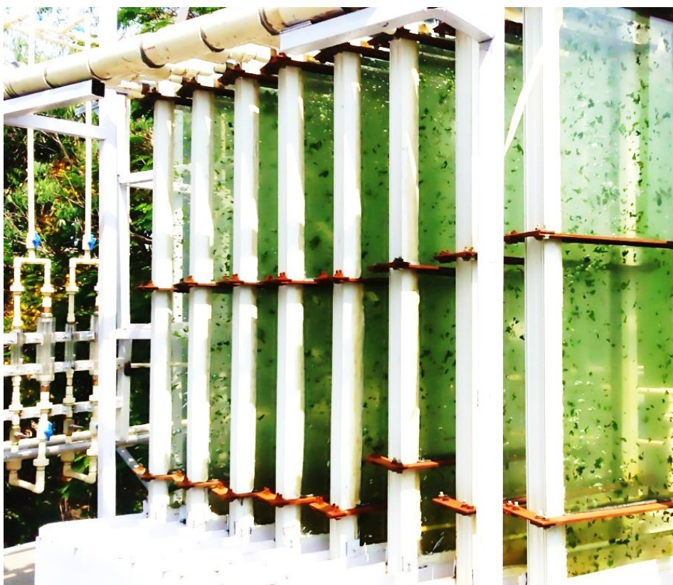
Fig. 1. Pilot scale flat panel photobioreactor for cultivation of sea-lettuce a.k.a. Ulva lactuca at DBT-ICT Centre for energy biosciences, Mumbai, India.
