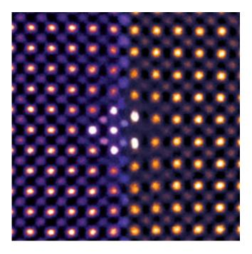
Colorized transmission electron microscopy of ceria ultrathin film reveals that individual atoms (shown as dots) shift under intense pressure. (Image credit: Sang Chul Lee)
