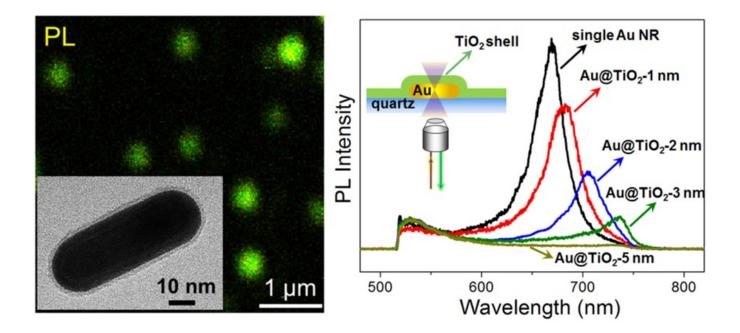
Early efforts to understand the emission from gold nanoparticles have relied on ensemble measurements. However, the chemical synthesis of metal nanostructures often yields a broad distribution of sizes, shapes, and constituents. Thus, single-particle analyses are essential to exclude undesirable effects caused by sample heterogeneity and impurities.
