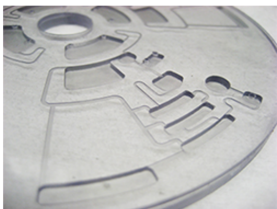
Fig. 1. A quadrant of a centrifugal microfluidic device made from clear polycarbonate plastic.
