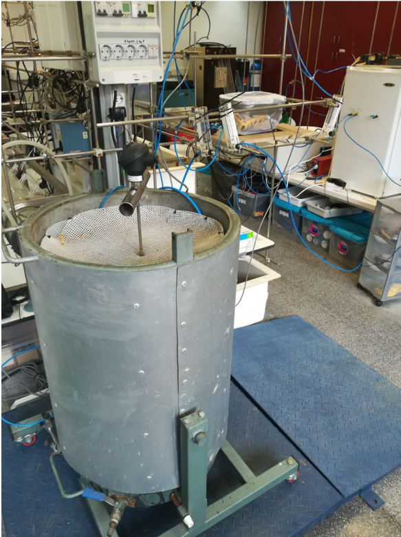
Fig. 2. Pilot plant for the study of gaseous emissions from biodrying of sewage sludge.
