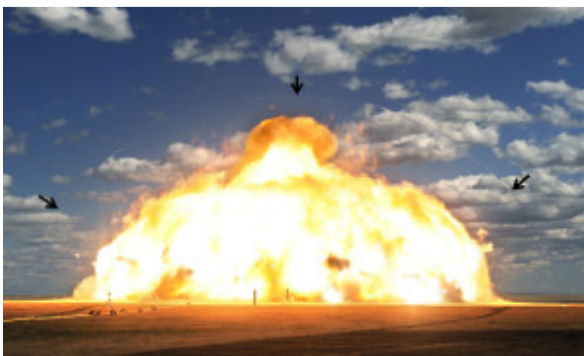
Fig. 1. A blast wave (arrows) is an area of pressure expanding supersonically outward from an explosive core. It can cause injury outside the area where an individual could be injured due to projectiles or being thrown.
