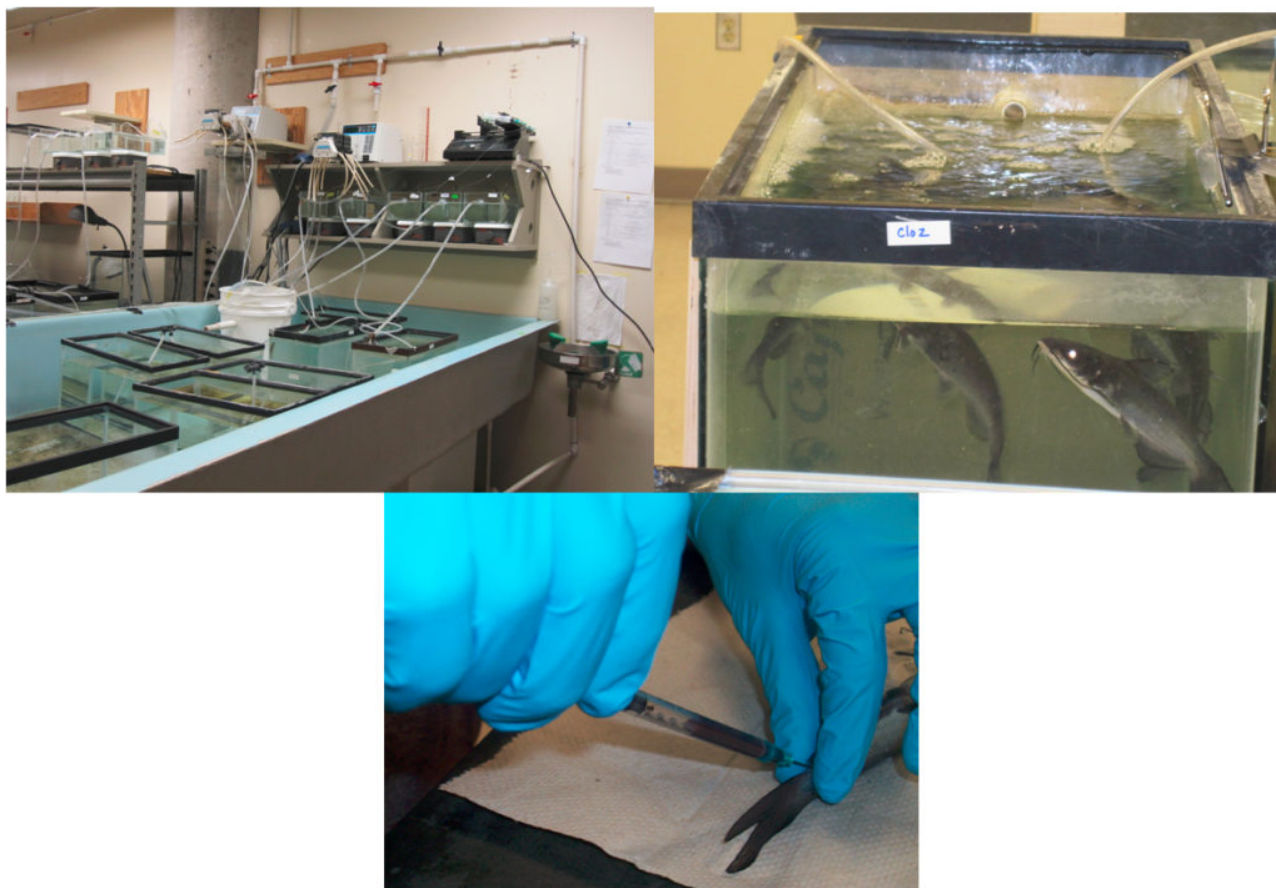
Bioconcentration testing with channel catfish. Top left - fish flow-through system; Top right -
