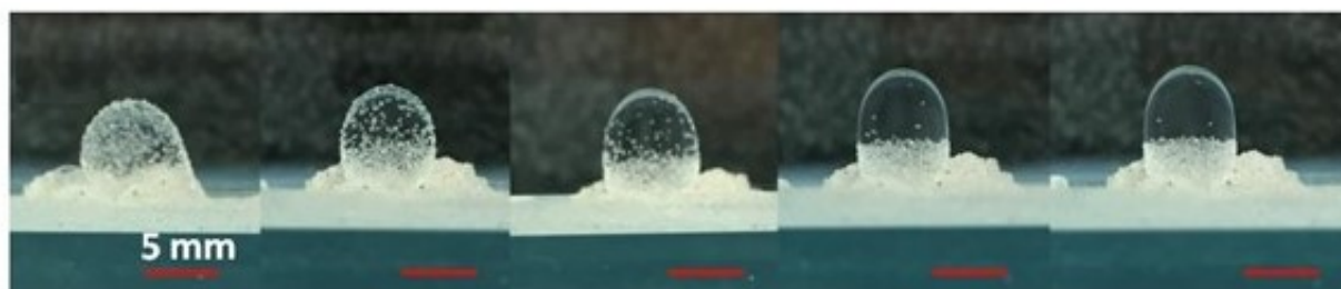
Fig. 1. Shape transformation of oil sack after stabilization of the encapsulation (silicone oil: viscosity 100 cSt, sand grain size 0.28 mm).
