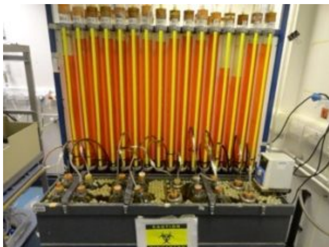
Fig. 2. Biomethane potential reactor.
