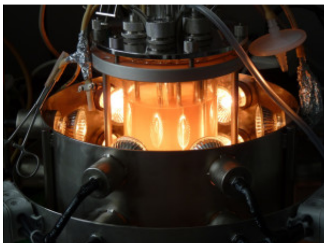
Fig.1. Continuous operated Halogen-photobioreactor using Rhodobacter sphaeroides DSM 158 for the photofermentative hydrogen production.
