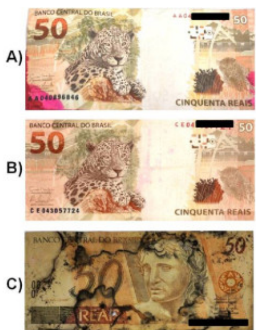
Fig. 1. A picture of one banknote each from the three sets of true forensic samples of seized banknotes with different ATD contamination: A) banknote recognized to be from an exploded ATM, presenting apparent ATD dye on the surface; B) banknote suspected to be from an ATM explosion followed by ATD impregnation, presenting characteristics of an attempted cleanup procedure with the use of organic solvents; C) banknote impregnated with a dark substance probably due to an attempt at cleanup using oxidative methods and/or high temperatures.
