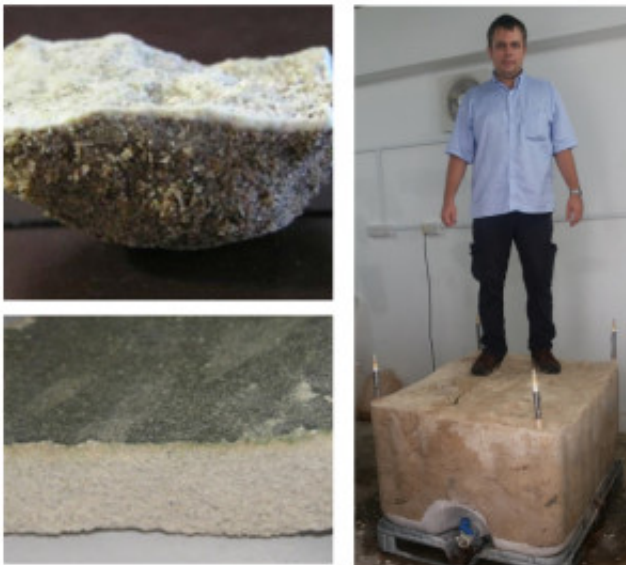
Fig. 1. Different types of biocemented structures in sand: calcite crust of sand surface, a layer and a block of biocemented sand.
