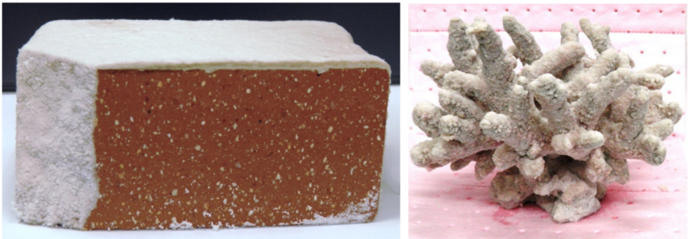
Fig. 2. The calcite-coated brick (“marble brick”) and the artificial coral, which was biocoated to facilitate formation of natural-like artificial coral reef.
