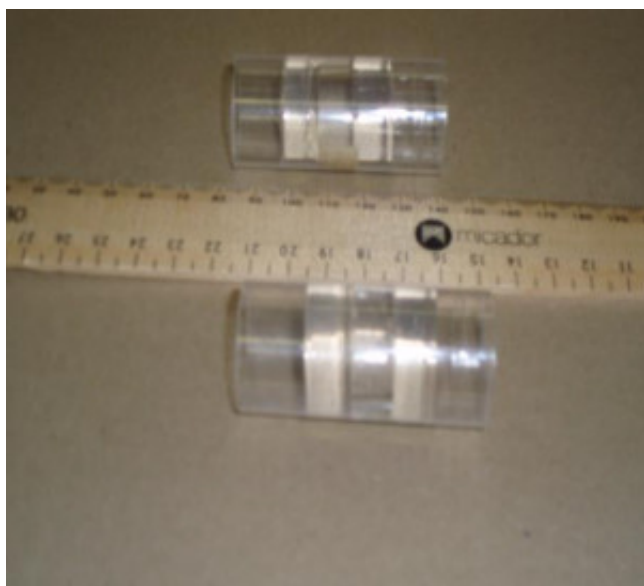
Fig. 1. 'Artificial mussel' device used in trace/heavy metals monitoring in Bangladesh (Kibria et al., 2012).
