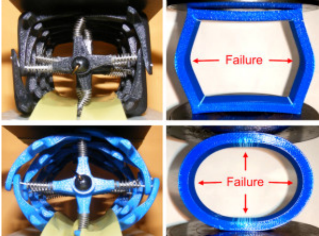
Fig. 2. Comparison of the square and circular prototypes (left) versus the solid rings without overlapping joints (right) subjected to compressive loading.
