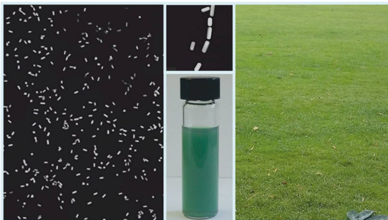
Fig. 1. TEM images of Ag nanorods (dark field imaging), a colloidal sample of the Ag nanorods solution and grass.
