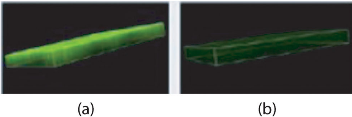
Fig. 1. A slice of an alginate hydrogel film showing penetration of fluorescent liposomes into the film (a) with ultrasound exposure and (b) without ultrasound. The film thickness is approximately 120 micrometers, and the film is covered by a liposome suspension. (From Ma et al., J. Acoust. Soc. Am., Aug 2015).
