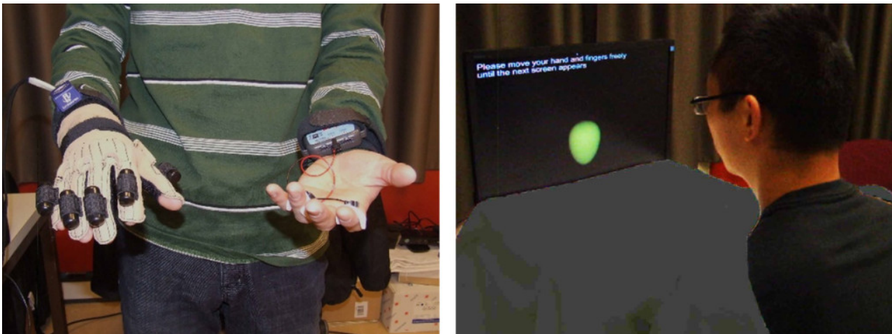
Fig. 1. Participants (Left) wore an orientation tracker and a data glove on their right hand, (Right) which was covered by cloth and a wooden box, and they saw a virtual balloon that they could make grow or shrink by opening or closing their hand, accordingly. The figure shows Ke Ma, the first author of the cited article.
